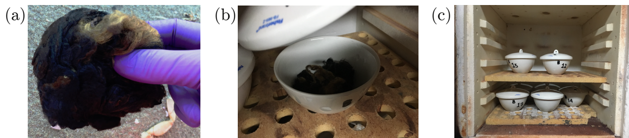
Figure 4: (a) MnO 2 impregnated acrylic fibers used in this study, (b) The ashing process showing one clump of MnO 2 impregnated acrylic fiber in a container ready for ashing and (c) samples in a muffle furnace prior to ashing.
