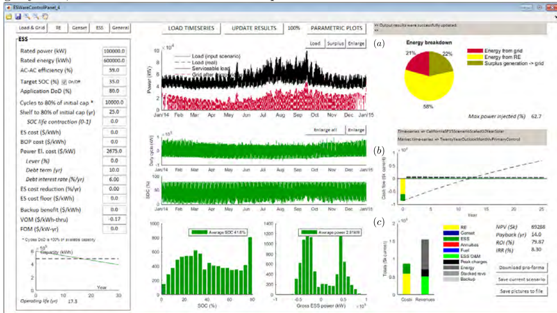
Figure 29: Characteristics of a system with PV renewable power generation, pumped hydro energy storage system, and collocated reverse osmosis plant
