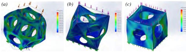
Fig. 3. von Mises stress results for vertical loading of a (a) dodecahedron, (b) octahedron, and (c) cube shell enclosure.
