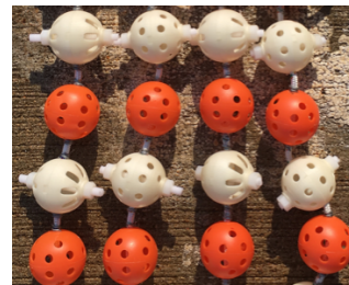
Fig. 6 Small section of net with white shells for adsorbent fibers. Adsorbent enclosure shells were alternated with orange placeholder shells used for mechanical testing.
