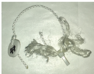
Fig. 9 Pre-weighed adsorbent mini braid. One to two of these mini braids were placed in each shell design on each of the two prototypes.
